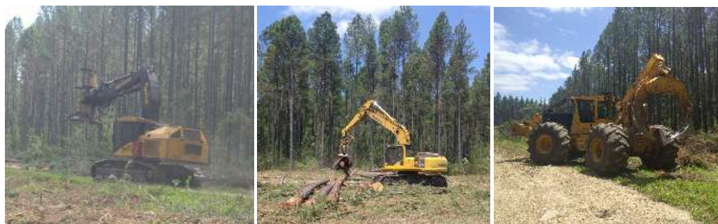
Figure 3. Whole Tree Harvesting System: (left) Feller Buncher, (centre) Processor, (right) Grapple Skidder
