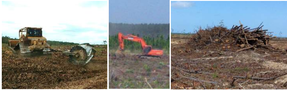
Figure 4. Site Preparation Operational Activities: (left) Chopper Roller, (centre) Excavator conducting CTL windrow, (right) Roadside pile after excavator manipulation prior to burning.
