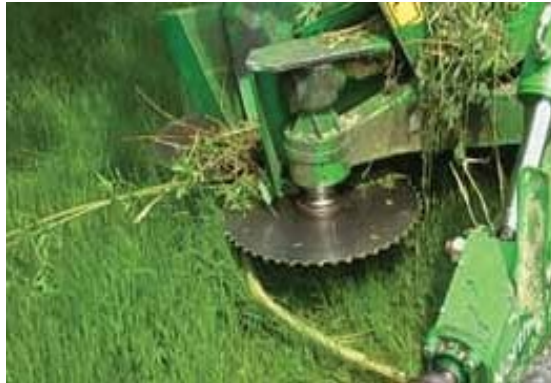
Figure 20: Harvesting head of Stemster rod harvester (Northern BioEnergy Ltd.Cookstown)
