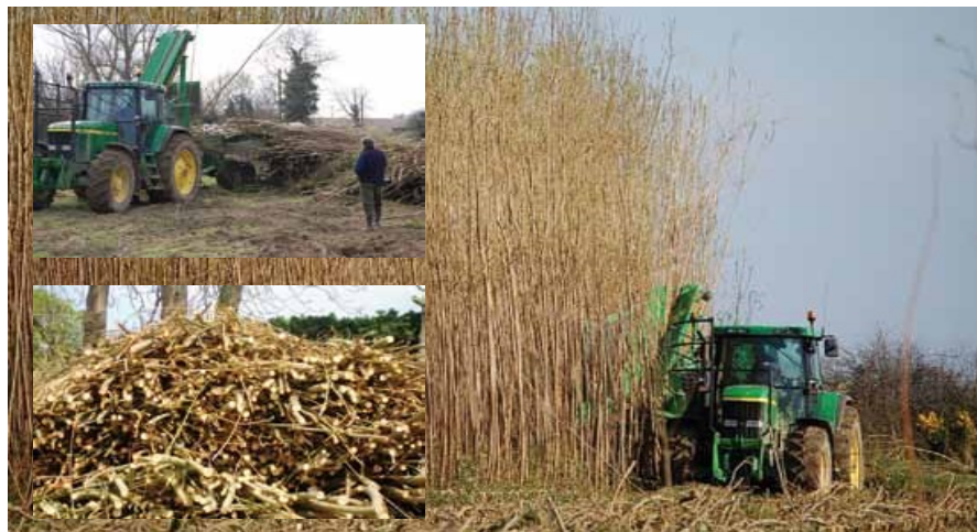
Figure 21: Stemster rod harvester working in three year old coppice, Drogheda. Insets Off-loading harvested rods and field drying rods. (Northern Bioenergy Ltd Cookstown)
