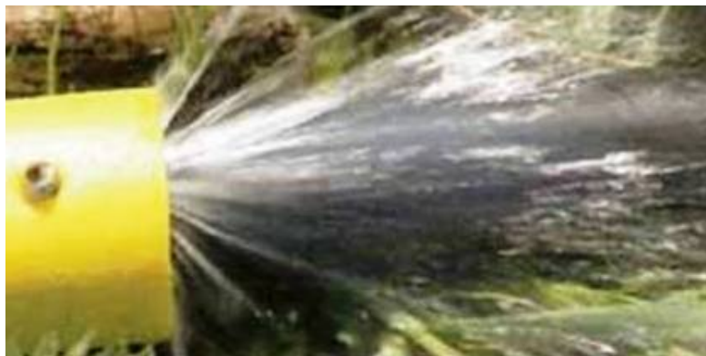
Figure 38: Detail of irrigation nozzle (Rural Generation Ltd)
