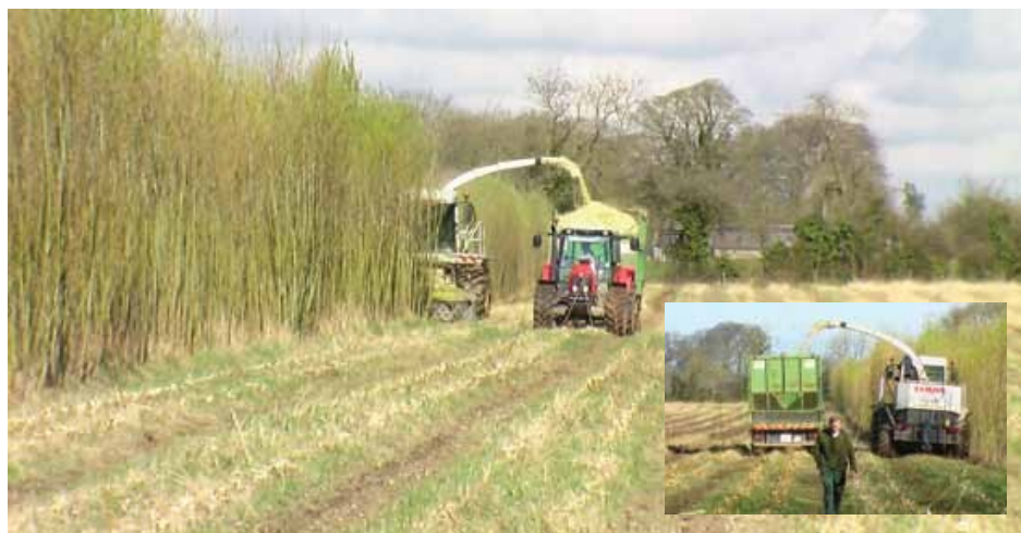
Figure 18: Class Jaguar direct chip harvester Co Wicklow (Sligo IT)
