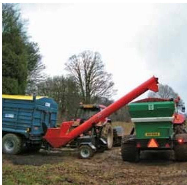
Figure 34: Loading sewage sludge from a sealed trailer through a closed auger to applicator. (Rural Generation Ltd)
