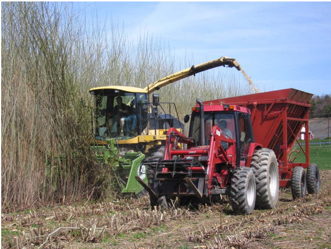
Figure 4: New Holland FX45 forage harvester and a specially designed hydraulically driven willow cutting head (CRL) from Coppice Resources Ltd in the United Kingdom was the first effective willow harvesting system in NY (photo by Lawrence Abrahamson).
