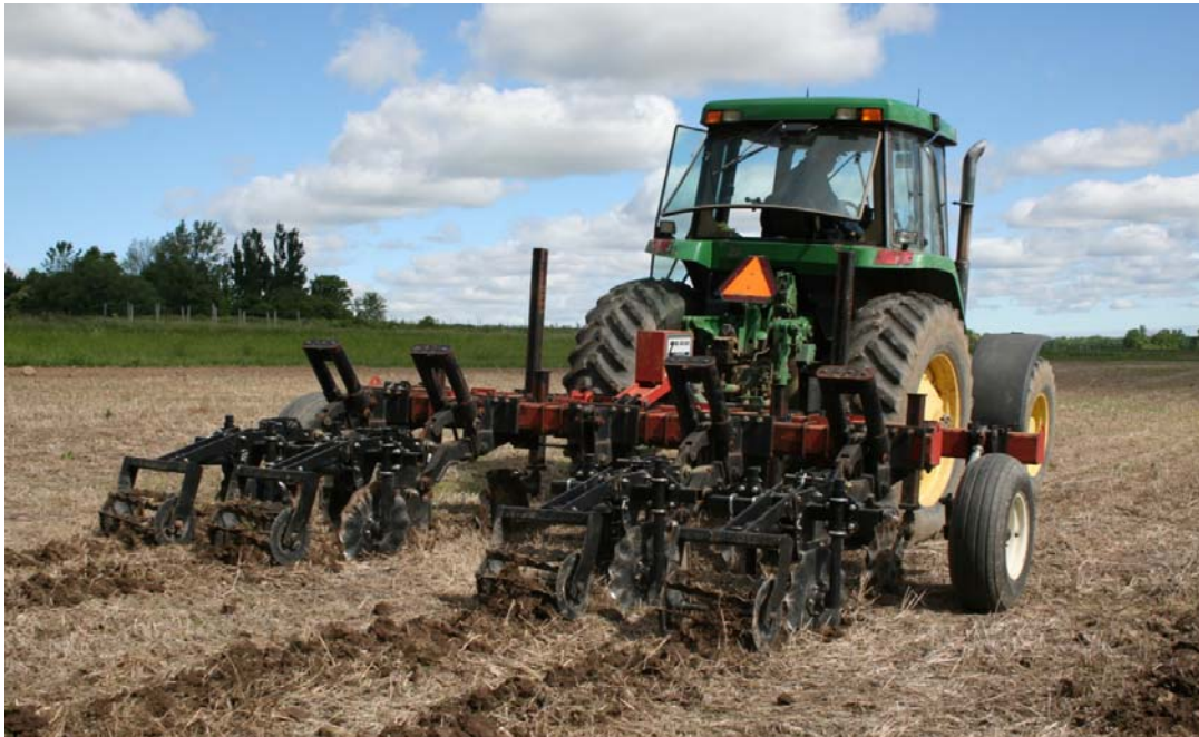
Figure 2: Zone tillage as an alternate site preparation method for willow bioenergy crops (photo by Lawrence Smart).
