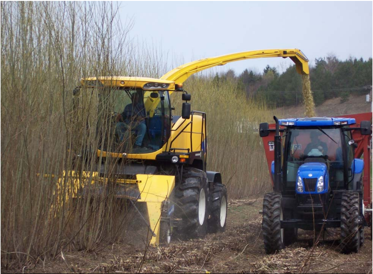
Figure 5: New Holland FR9080 and New Holland 130FB coppice header harvesting 3-year old shrub willow in Tully, NY during Spring of 2010 (photo by Lawrence
