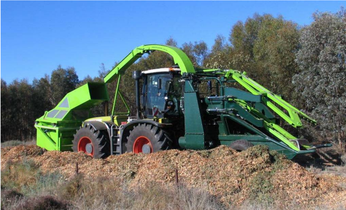
Figure 3. A pre-commercial mallee harvester during trials conducted in Southern Australia. Significant resources from industry and government are committed to the development of a harvester that is capable of efficiently harvesting native Australian species and chipping the biomass in-field (image: R. Giles).
