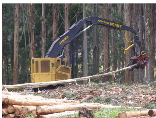
Figure 4.2: Tigercat tracked harvester delimiting and topping a felled Eucalyptus nitens stem during a streamside harvesting study on the effectiveness of Best Management Practices. Note the slash coverage remaining in the harvested area. Photo credit: Daniel G. Neary
