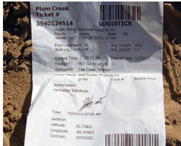
A timber harvest load ticket used to track harvested wood in Georgia’s fiber market.
