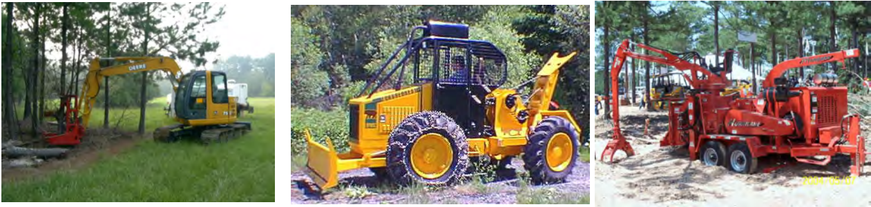
Figure 5. Harvesting system including small feller-buncher, mini-skidder and chipper in South USA (O’Neal and Gallagher, 2008)
