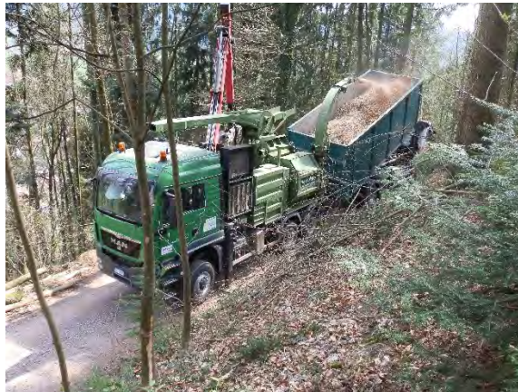
Figure 12. Truck mounted chipper working at road side in mountainous forests in Italy (Spinelli, 2015)
