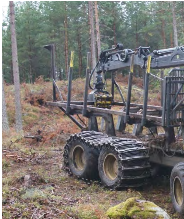
Figure 16. Modified bin load of a forwarder to extract residues in Sweden. Note the framework on the bunks and the rearward extension with the two slightly rearward leaning additional rear posts. (Eliasson et al. 2011)
