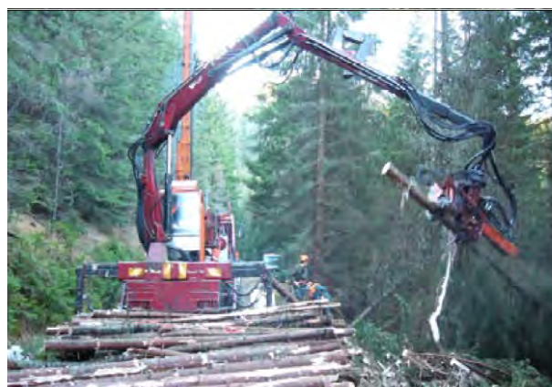
Figure 6. Wanderfalke tower yarder combined with a processor at road side (Austria) (Affenzeller and Stampfer, 2007)
