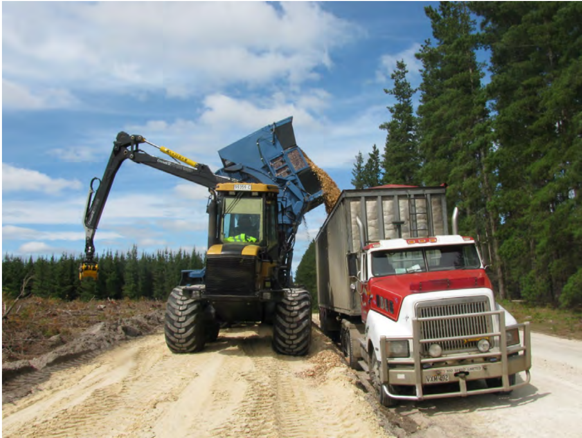
Chipping operations by a mobile chipper in pine plantation in Victoria (Australia)
