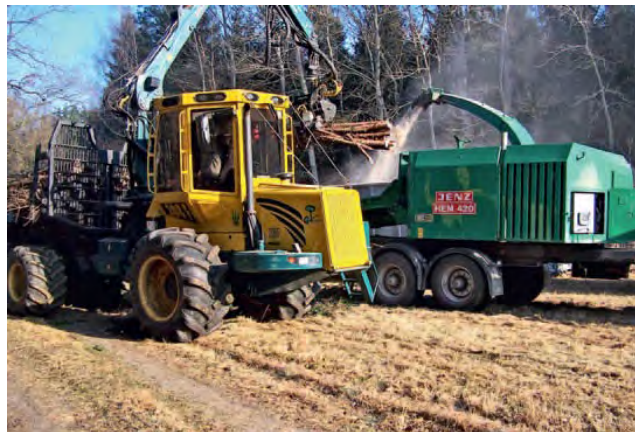
Figure 10. Chipping energy wood by Jenz HEM chipper in Germany (KWF, 2012)
