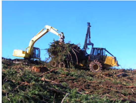
Figure 3. Forwarding harvesting residues by a forwarder in Northwest USA (Sessions, 2015)
