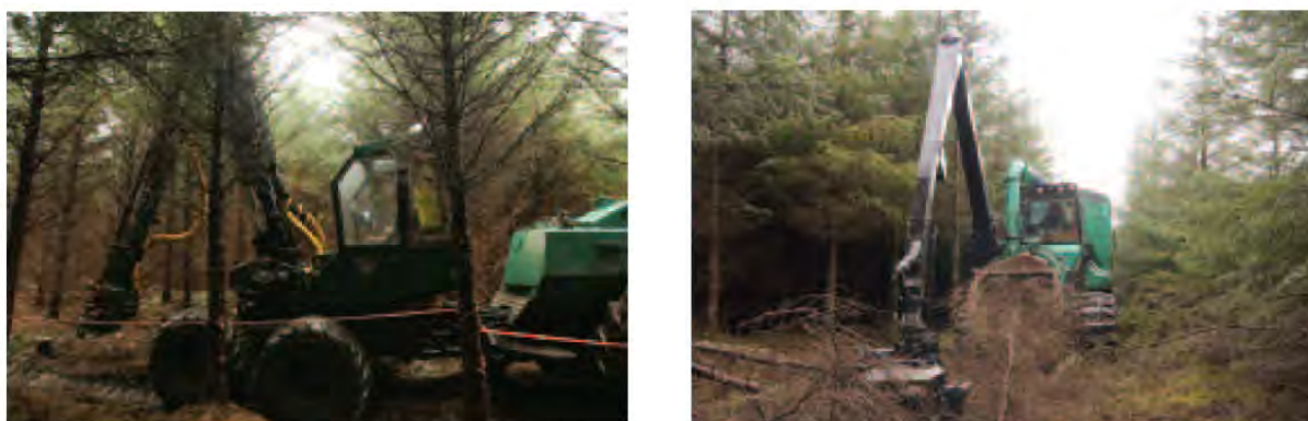
Figure 7. Whole tree chipping by combination of feller-buncher and chipper in Denmark (Kofman and Kent, 2009)
