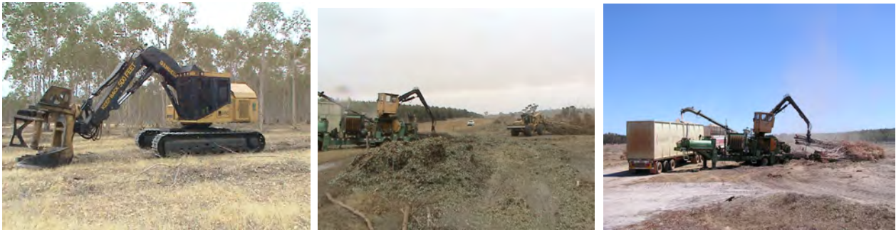
Figure 19. Whole tree chipping operations in Eucalypt plantations in Western Australia
