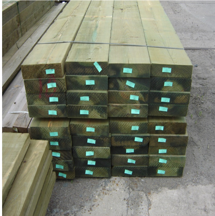
Figure 67. Pressure treated beams used in residential and commercial construction. (Photo courtesy of Oriental Lumber, New York)
