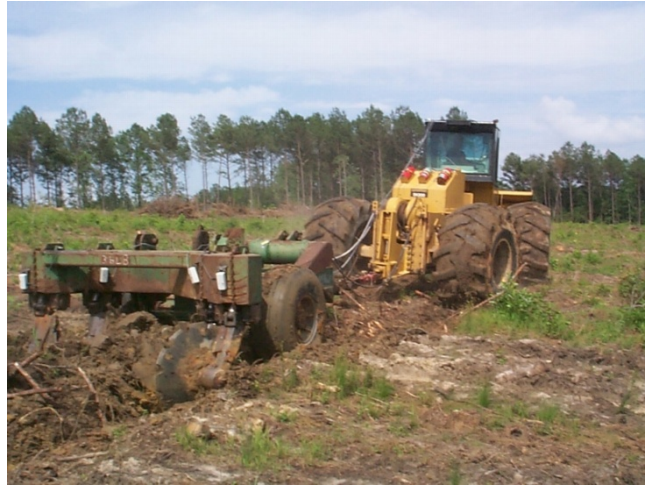
Figure 40. Site preparation discing and bedding operation, Alabama, USA (Photo courtesy of the USDA Forest Service and Auburn University).
