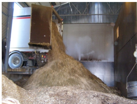
Figure 64. Delivery of wood chips to a small bioenergy producer (a) for storage (b) prior to utilization for energy production, Joensuu District, Finland. (Photos by Daniel G. Neary).
